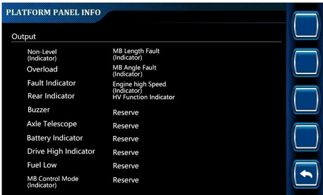
Fig. 37 PLATFORM PANEL INFO interface-output
