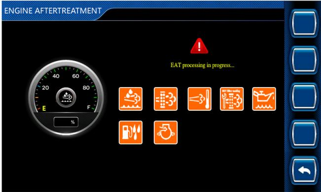
Fig. 32 EAT INFO interface (with EAT started)- Equipped with Deutz engine
