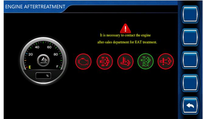
Fig. 33 EAT INFO interface (with EAT started)- Equipped with Yuchai or Yanmar engine
